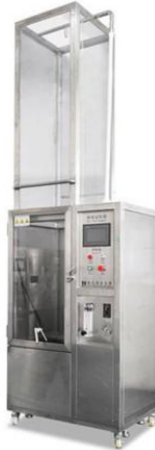
IPX5/6 Flushing Test Equipment (φ6.3mm, φ12.5mm Nozzle)
